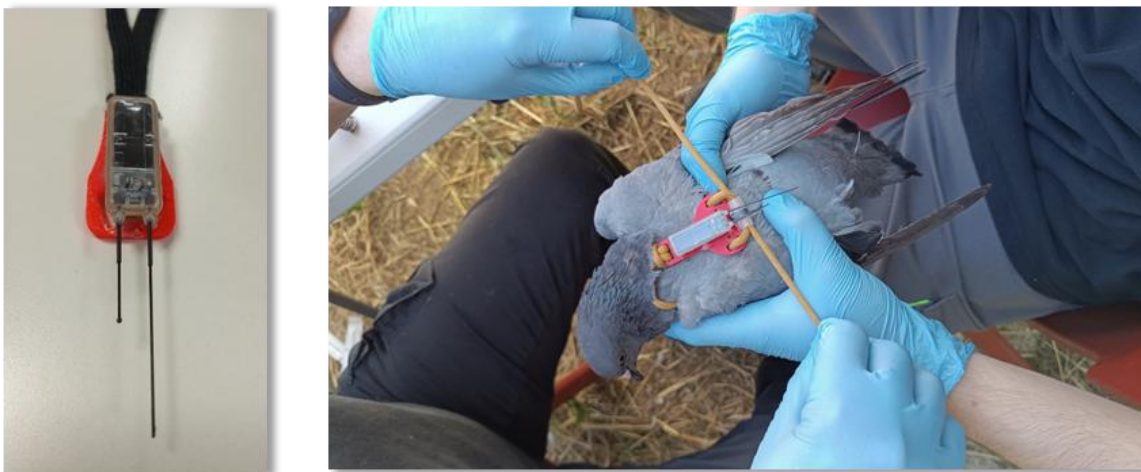
Figure 1. GPS device attached to the harness and technicians placing the assembly on a pigeon.
