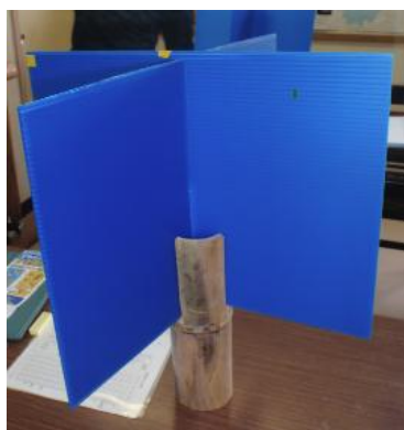
Figure 3. Directional sticky-board trap, which is a blue colored board (30 × 23 cm) with an improved flight interception trap.
